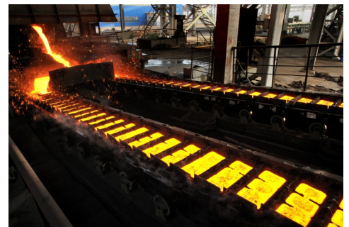
Fig 2: conveyor belt with molds
