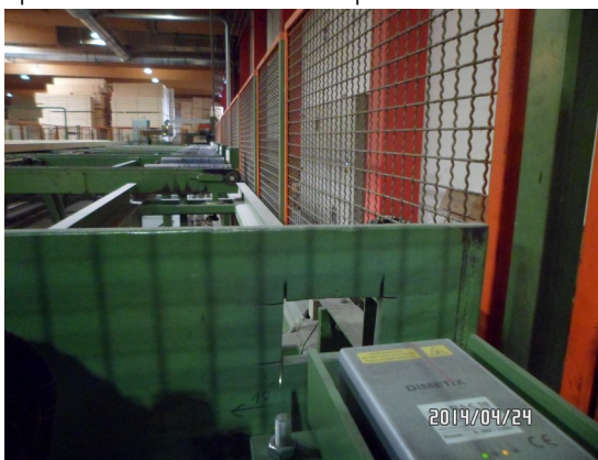
Fig 1: Dimetix Laser measures the wood face-on
