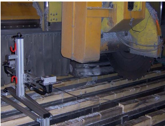
Fig 1: Gantry saw with Dimetix Laser
