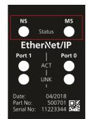
The status LED's of the EtherNet/IP<sup>™</sup> protocol are marked in figure 11. The possible EtherNet/IP<sup>™</sup> status conditions are displayed with two green and two red status LED's with three LED states – OFF, ON or FLASHING.
