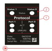
Identification of the existing status LED's of the exchangeable cover with Industrial Ethernet:
