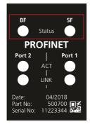
The status LED's of the PROFINET® protocol are marked in figure 10. The possible PROFINET® status conditions are displayed with two red status LED's with three LED states – OFF, ON or FLASHING.
