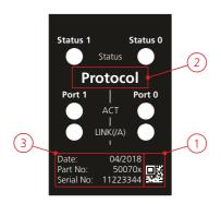
Identification of the exchangeable cover with Industrial Ethernet:
