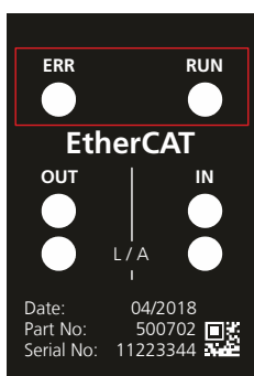
Figure 12: EtherCAT® status LED's
