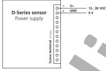
Figure 7: Connection of power supply (V+ and GND)
