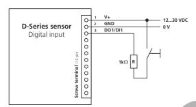
Figure 12: Connection of digital input for external triggering
