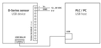
Figure 19: Connection of USB interface
