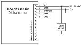
Figure 11: Connection for digital output (DO1, DO2, DOE)
