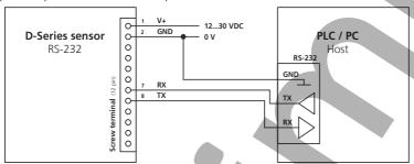
Figure 14: Connection of the RS-232 interface
