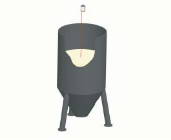
Level measuring of silos
