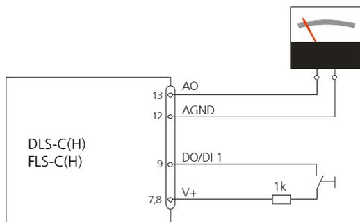
Fig. 5: Use digital input as external trigger
