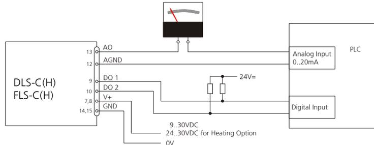
Fig. 17: Connection of an instrument and a PLC
