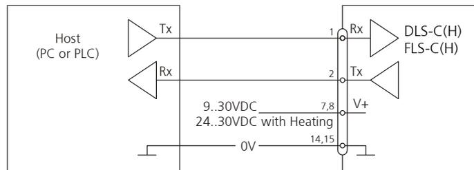
Fig. 15 Point-to-point connection with RS-232
