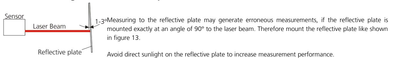
Fig. 13: Reflective Plate mounting
